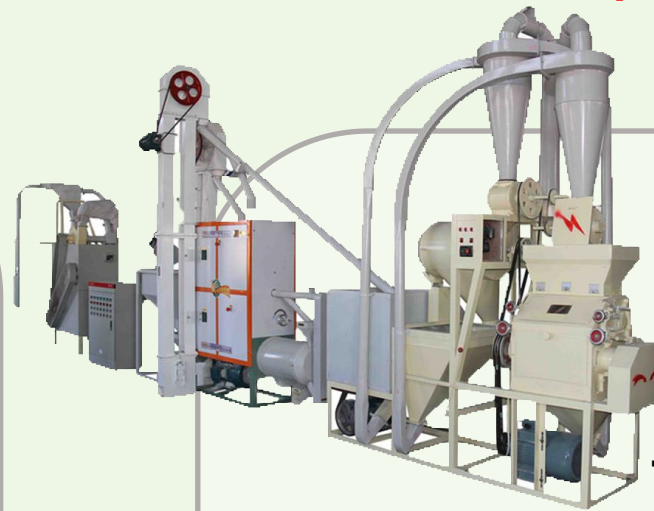
6FW-8AB 8TPD Corn grits and flour milling line
