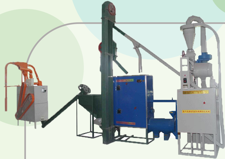
6FW-8AB 8TPD Corn grits and flour milling line
